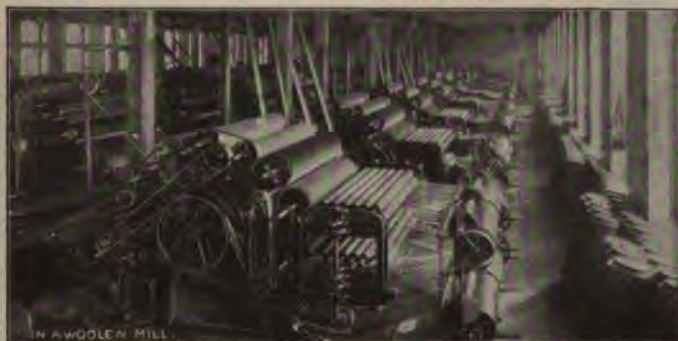
Wool-carding machines at Lawrence, Mass. They straighten the fiber and separate it into long rolls that are next drawn out and twisted into yarn.
